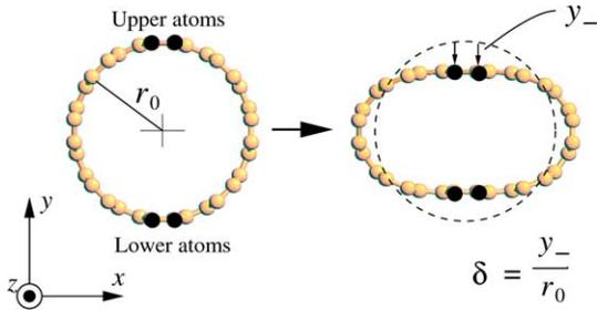
Fig. 2. Radial compression of CNTs.
