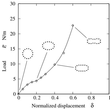
Fig. 3. Change in load of (8,0) CNT under radial compression.
