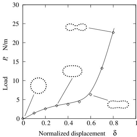
Fig. 4. Change in load of (12,0) CNT under radial compression.
