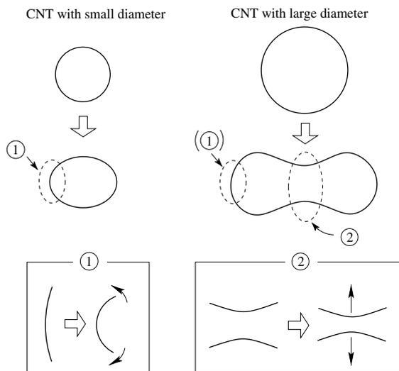
Fig. 6. Deformation mechanism of CNTs under radial compression.
