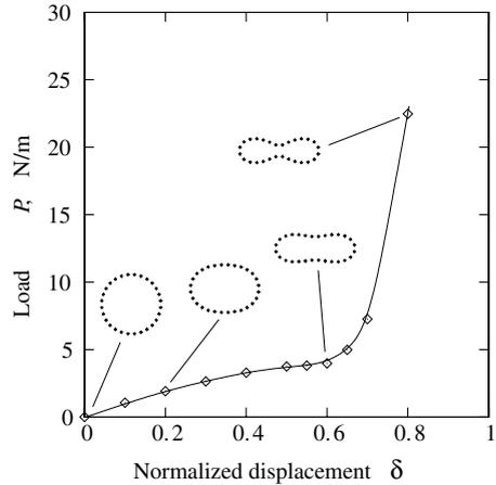
Fig. 5. Change in load of (14,0) CNT under radial compression.
