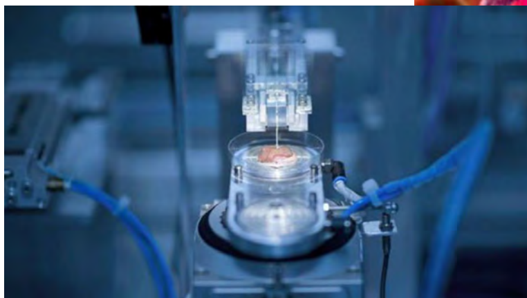
The system that can rapidly manufacture two-layer artificial skin models.
